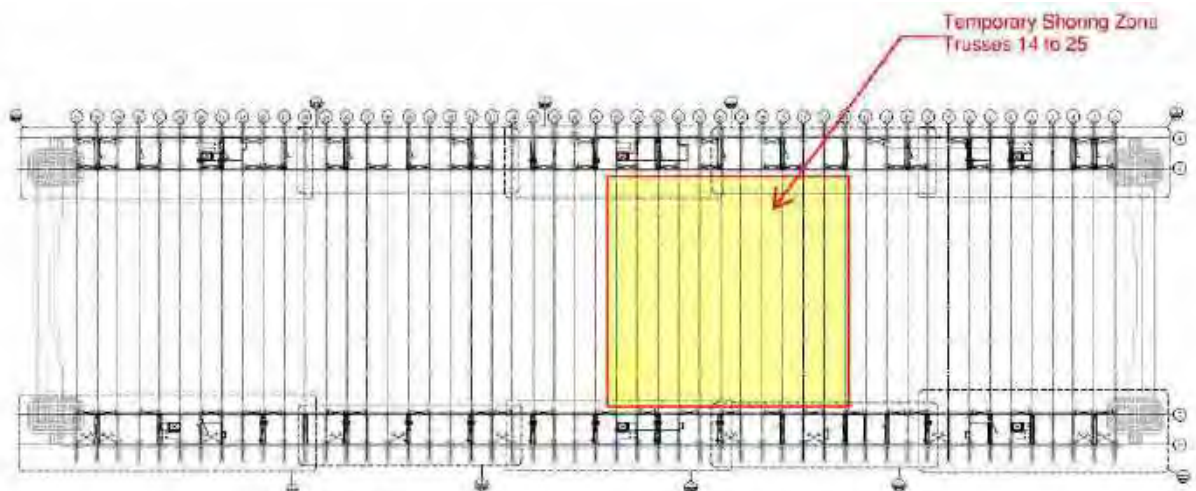
Figure 12. Zone of temporary shoring.
